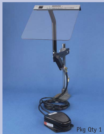
No. SPU4M01 Extra Heavy Duty T-End™ Industrial Tool with benchmount & foot pedal actuator
